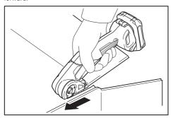
**NOTICE:** Do not apply excessive force to the tool. It does not help to cut the material smoothly.
