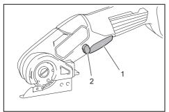
1. Switch trigger 2. Lock-off button
